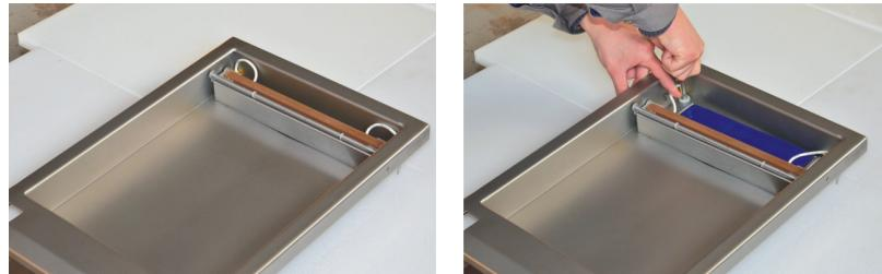
1. Disconnect the cable from the pin, then pick the complete sealing bar up from the vacuum chamber.
