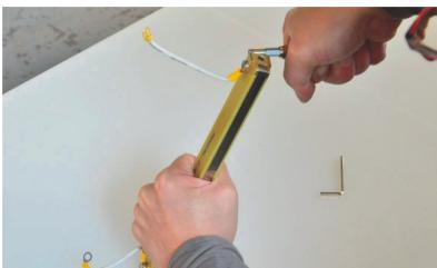
7. Fasten the heating wire, then cut the excess heating wire.
